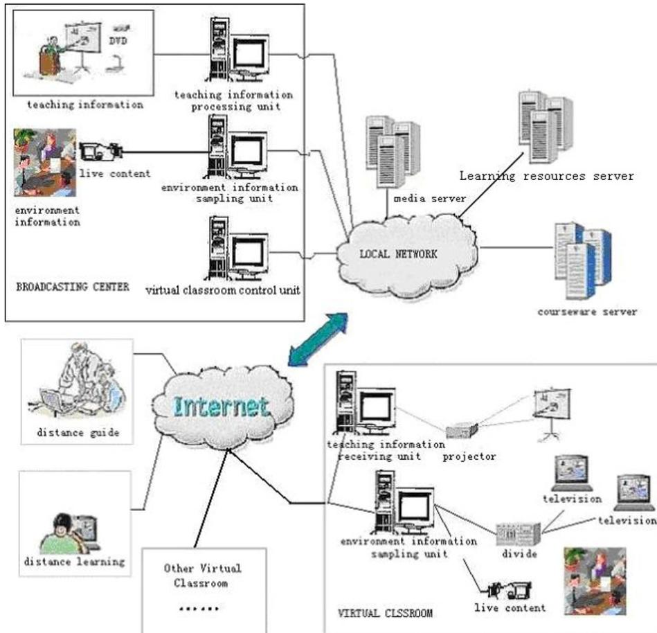
Fig. 1. WVOC is composed of broadcast center, virtual classrooms, and servers.
