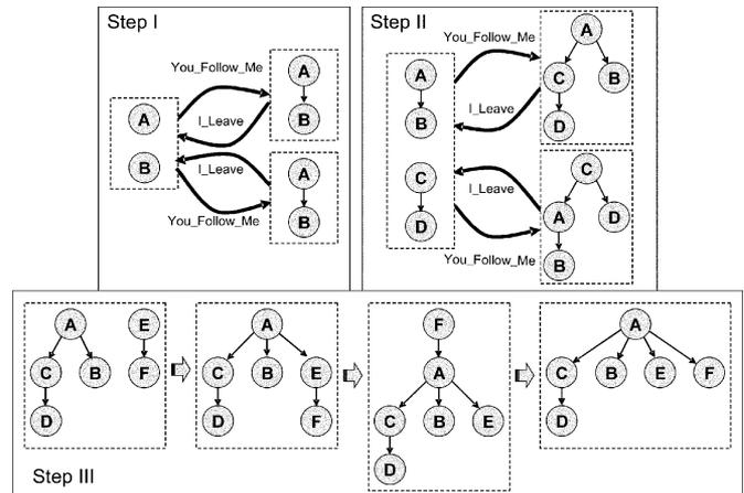
Fig. 11. SDTs generated during the prototype testing.
