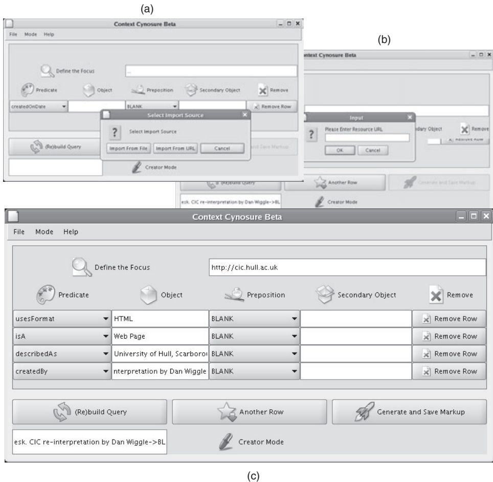
Figure 5: Process of importing Dublin Core metadata into the context model (a) Select import source. (b) Input the source's uniform resource locator. (c) Metadata is extracted and imported into the context model.
